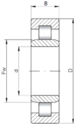
55 mm x 120 mm x 49,2 mm 55 mm x 120 mm x 49,2 mm ISO NU3311 cylindrical roller bearings
