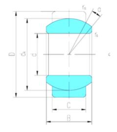
GE6E Bearing 2D drawings and 3D CAD models
