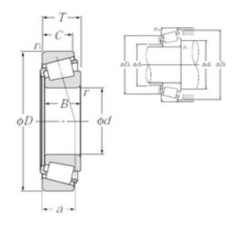
4T-L812148/L812111 Bearing 2D drawings and 3D CAD models
